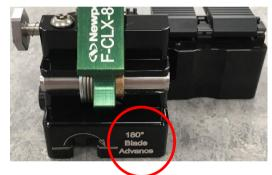
This is shown underneath by a scale printed on the blade advance block (see green circle). The blade is 3.5mm long and so there are up to 10 positions on each blade.
