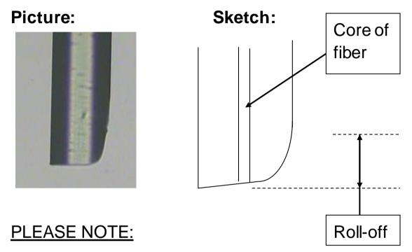
The angle of the core of the cleaved end cannot be measured by inspection from the side of the fiber. The core is not visible when viewed from the side of the fiber.
